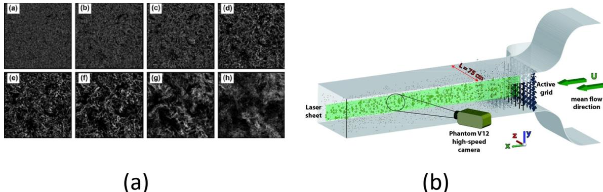
**Figure 1:** Illustration of the formation of clusters and voids from the simulations of Yoshimoto and Goto 2007 (a) and schema of the experimental set-up at LEGI (b).
